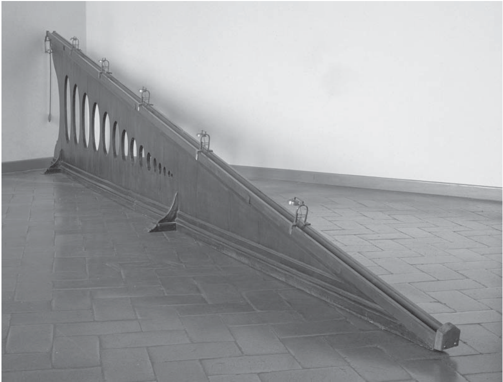
1 Inclined plane with catgut strings and bells used by Galileo, now in the Istituto e Museo di Storia della Scienza in Florence (© Photo Franca Principe, IMSS, Florence)
